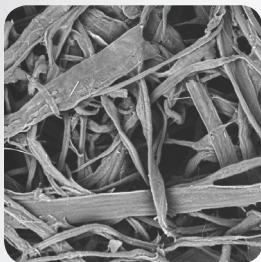
Magnification of 250x shows conventional cellulose filtration fibers and the spaces allowing larger particles to pass through to the engine.
