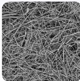
Magnification of 250x shows how Royal Purple's state-of-the-art synthetic filtration media provides greater filtration efficiency and particulate capacity while minimizing flow restriction.
